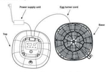
d, Place the top onto the incubator base lensuring the clear window is completely closed. It's important to align the two notches on the bottom of the clear window with the two sockets on the base.
