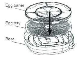
c) "Iug the egg turner cord (coming out from the bale) into the socket located on the back of the incubator top. Connect the power Lupply unit to the incubator top.
